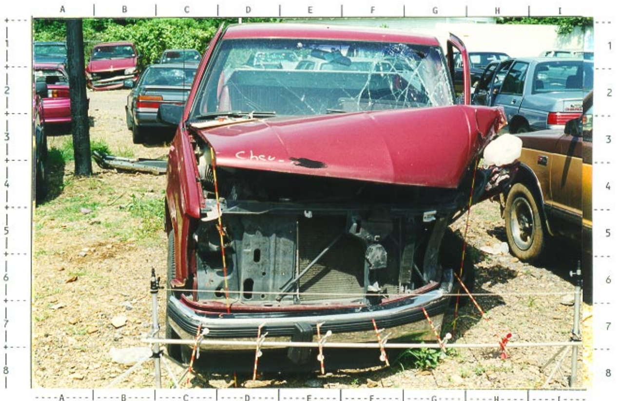
# 62 -- Frontal view of 1988 Chevrolet C-1500 pickup's front left damage with contour gauge present
